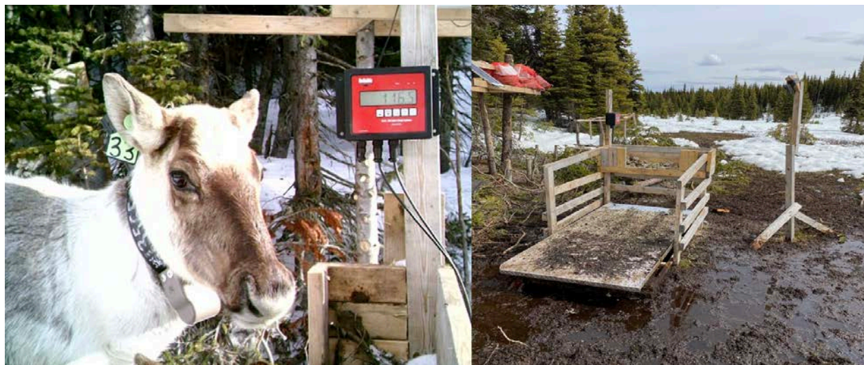
Figure 4. Caribou stepping on the scale can be identified by ear-tag combination, and the scale readout indicates their current weight
