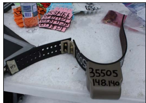
Figure 1. Vectronic GPS radio collars were fit on all adult caribou. Note the rot-away section on the left hand side, ensuring that if a collar stops working, it will not be permanently fixed to the animal
