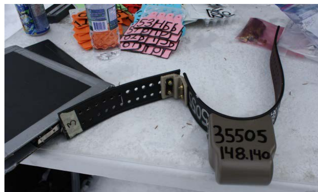
Figure 1. Vectronic GPS collars were fitted on all captured caribou. Note the rot-away section on the left hand side, ensuring if a collar stops working, that it will not be permanently fixed to the animal.
