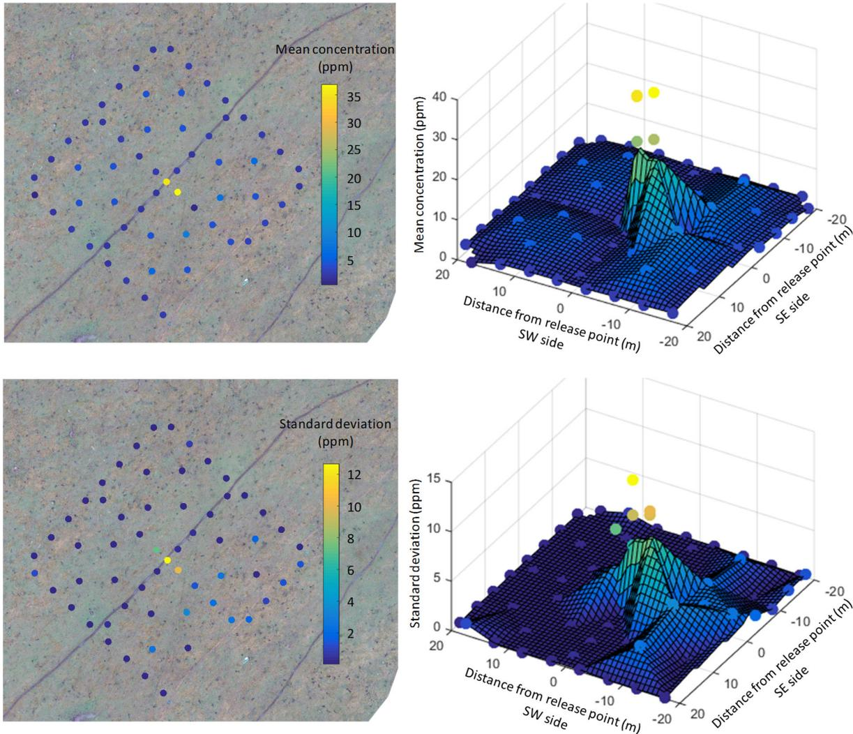
Figure 12. Plan and 3D view of mean and standard deviation of methane concentrations near the release point.
