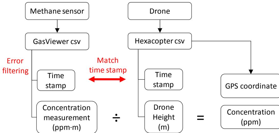
Figure 6. Data processing procedure.
