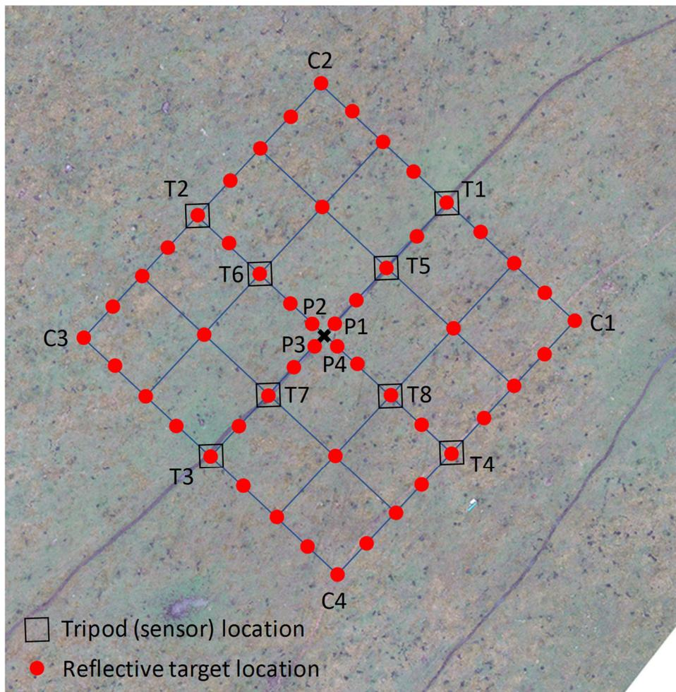
Figure 5. Layout of the ground-based measurement grid in the open field.
