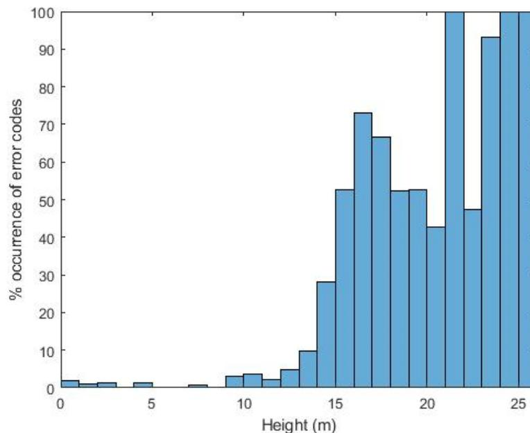
Figure 21. Sensor error code occurrence with drone height over grassy terrain.
