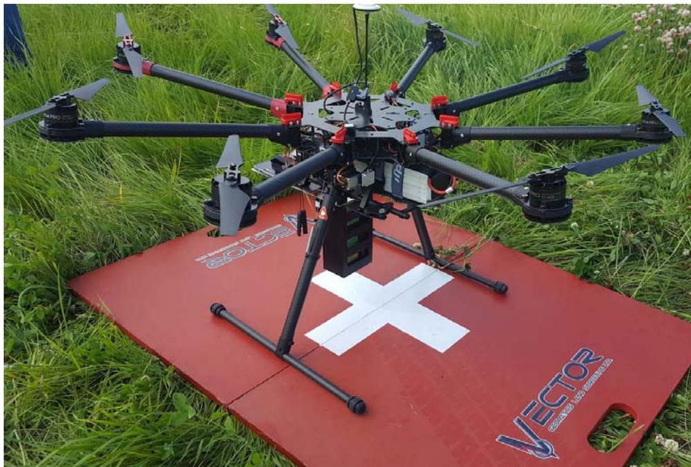
Figure 4. DJI Spread Wings S1000 with a Laser Methane mini-G sensor and Android phone mounted below.
