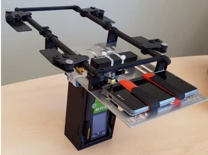
Figure 3. Vibration isolating mounting plate for the methane sensor and Android phone.
