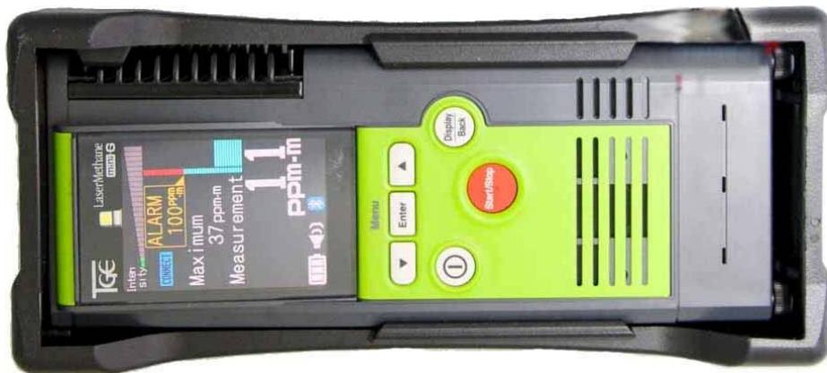
Figure 1. Laser Methane mini-G sensor.
