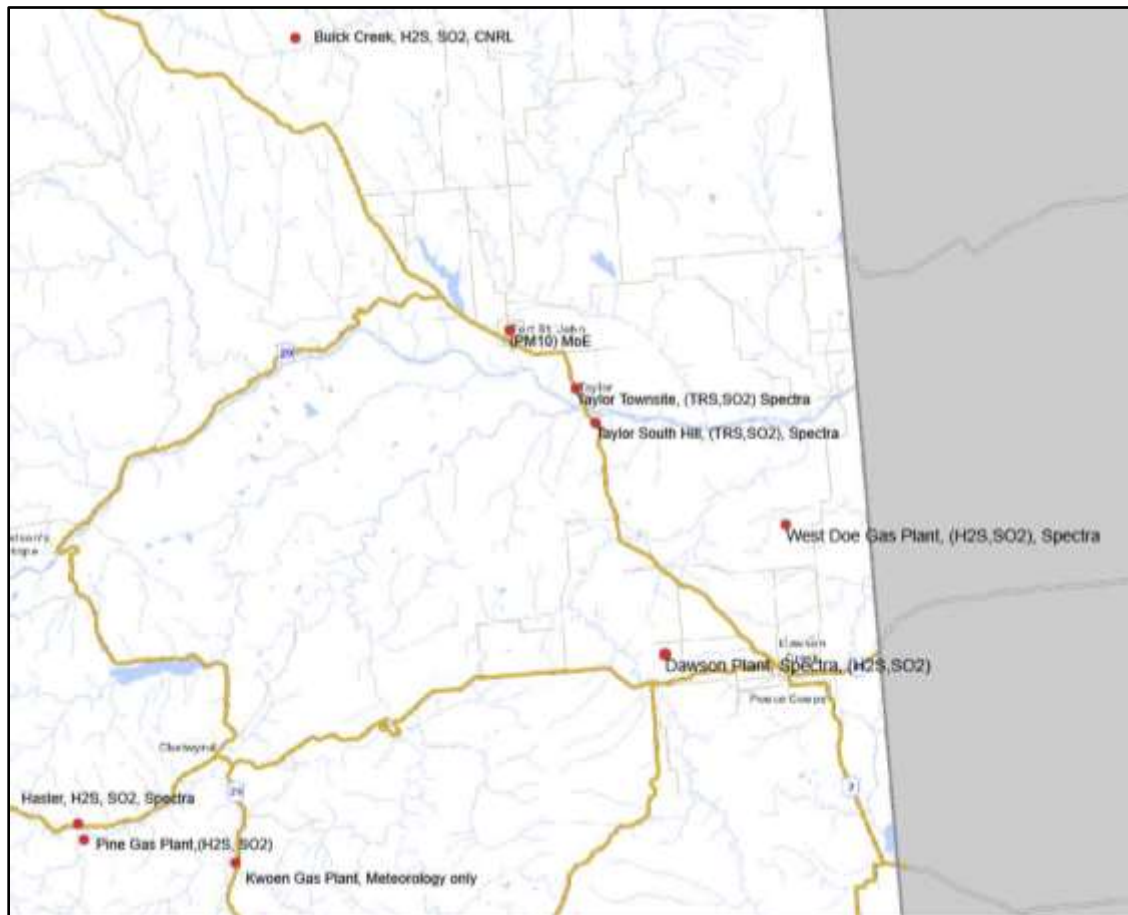
Figure 2 Hourly monitoring sites in the NE B.C. Air Quality Monitoring Network as of November, 2013. Pollutant concentrations measured by this network appear in real time on the website BCAirQuality.ca . The exceptions are Buick Creek, West Doe Gas Plant and Dawson Plant that are operated by industry. Historical data from 1992-2013 are also available to the public.
