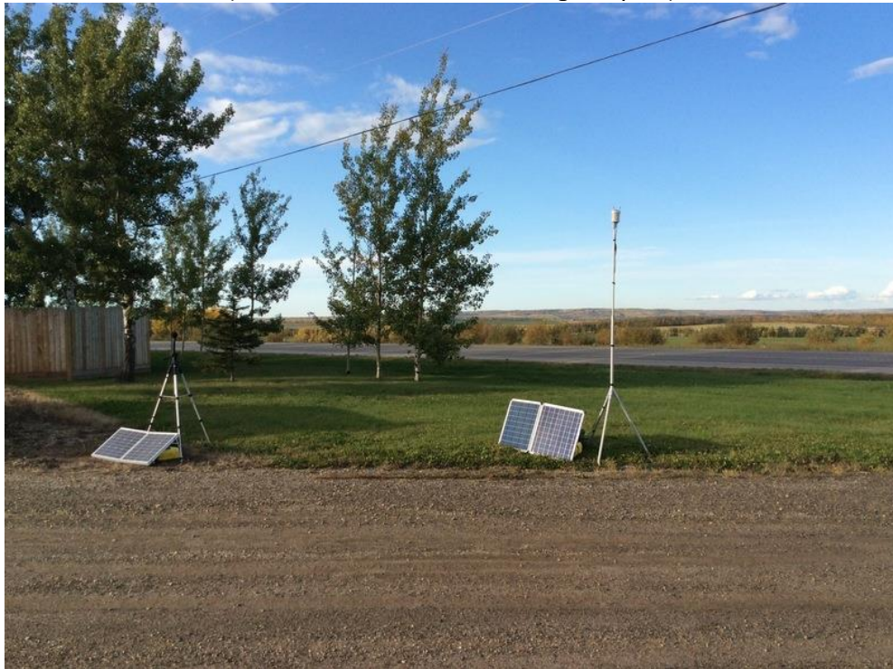
Picture C2: Sound Monitor C and Weather Monitor Setup (Southwest 20m from the Highway 97)
