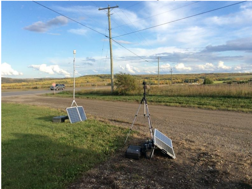
Picture C1: Sound Monitor C and Weather Monitor Setup (Southwest 20m from the Highway 97)
