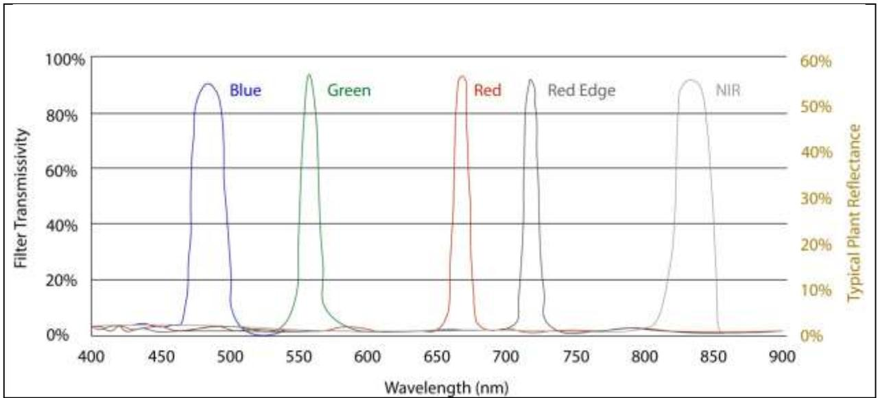
Figure 2: Sample of the band set for a popular (Red Edge from Micasense) MSS camera.
