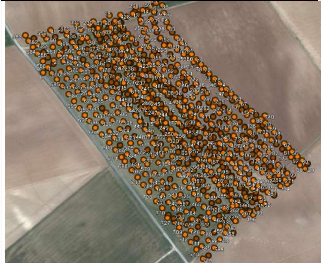
Figure 1. Sample of flight plan with triggering points for aerial photography. A high degree of overlap (side and edge) result in a relatively large number of photographs per project area.
