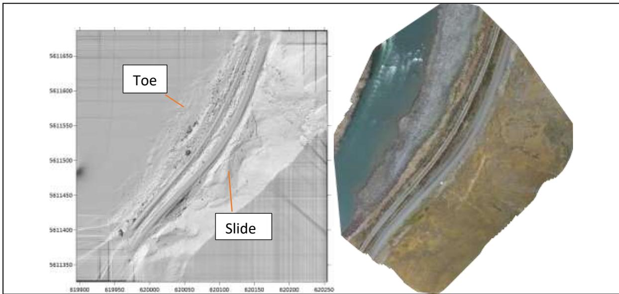
Figure 5. Sample of a DEM of a small landslide and the aerial photo mosaic of the same area. Both images were captured with UAV-based LiDAR and camera. (source: UVic HLRG)
