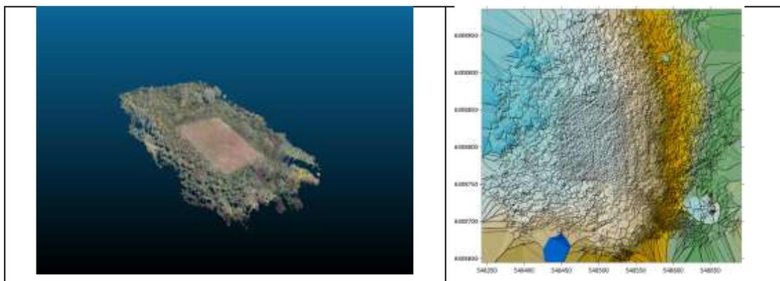
Figure 16. Point cloud perspective for Site 3 and bare earth DEM from the point cloud.
