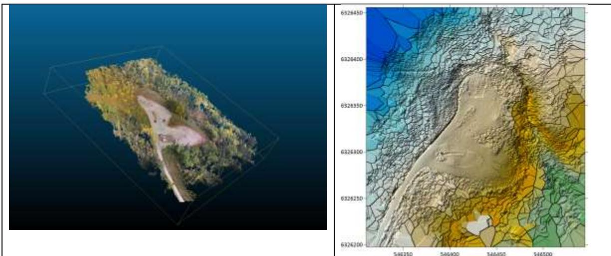
Figure 15. Site 2 SfM point cloud perspective view and a bare earth DEM (gridded to 25 cm) from this point cloud.
