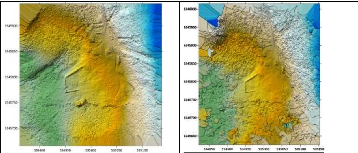
Figure 19. Comparison of the bare earth DEM derived from the LiDAR on left, with SfM point cloud on the right.
