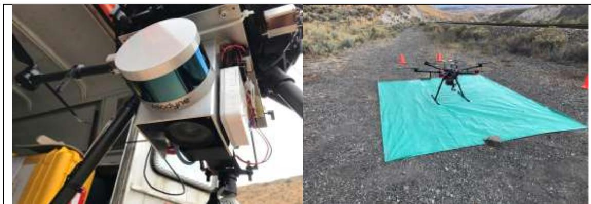
Figure 8 Configuration of the payload on the M600 and M600 ready to deploy.
