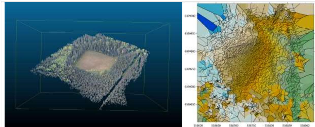
Figure 21. Perspective plot of the SFM point cloud on left and bare earth DEM from the point cloud on the right.
