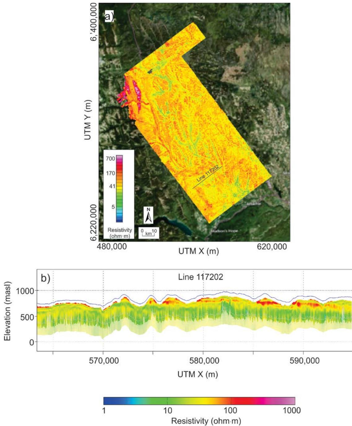
**Figure 6.** Interpretation results of the 1D inversion of AEM data collected from the SkyTEM survey for the Peace Project Main Area derived from laterally constrained inversion. a) Example of a horizontal subsurface resistivity slice showing the resistivity distribution from 6.8 to 9.7 m below ground surface at approximately 1:850,000 scale. b) Example of a vertical resistivity section showing the resistivity distribution along flight line 117202. Modified from SkyTEM Surveys ApS (2015).
