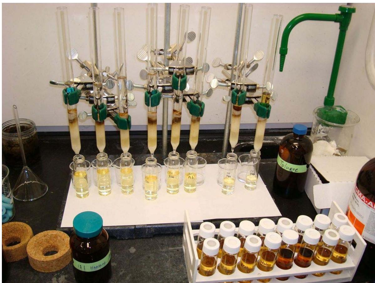
**Figure 3.9 Silica gel cleanup of PHCs in soil**
