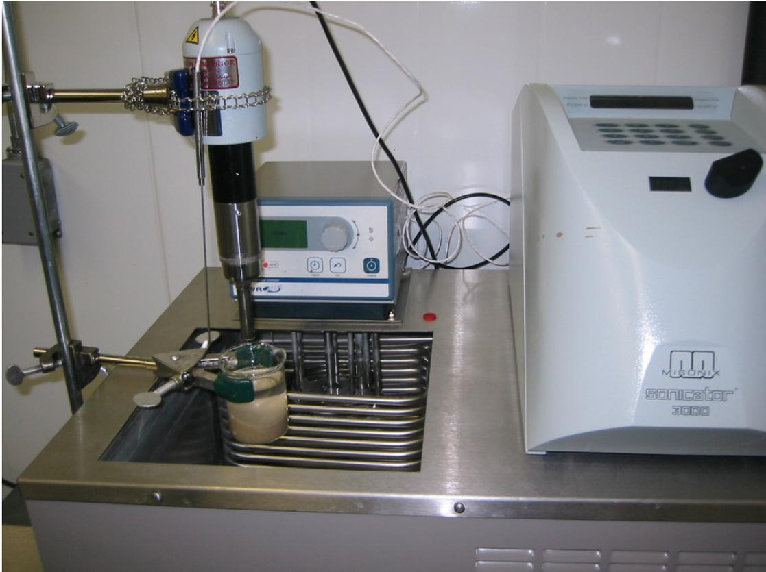
**Figure 3.2 Sonic probe and sample setup**
