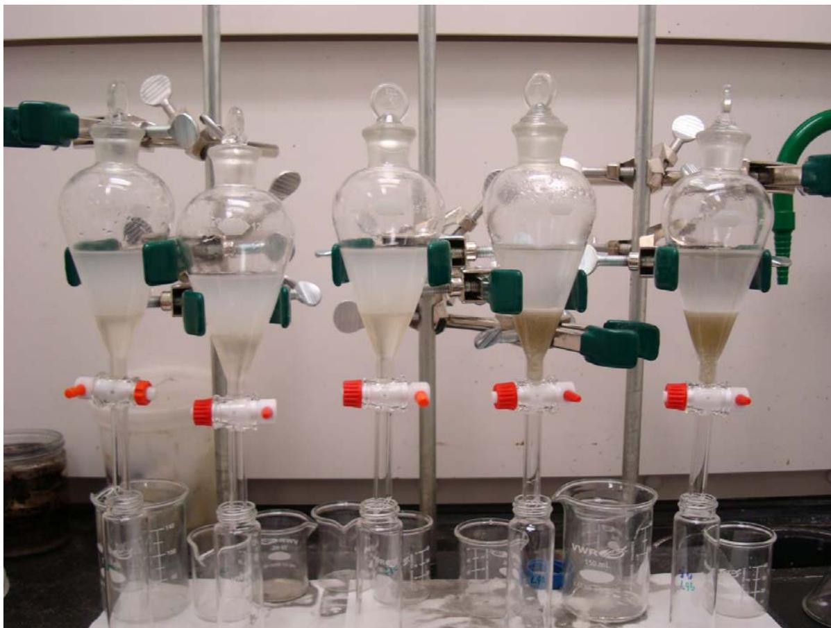
**Figure 3.8 Separatory funnel liquid – liquid extraction**
