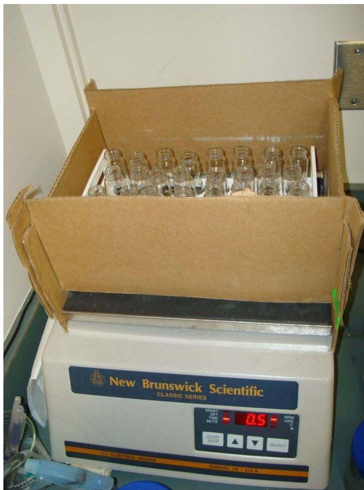
**Figure 3.7 Mechanical shaking for soil extraction**
