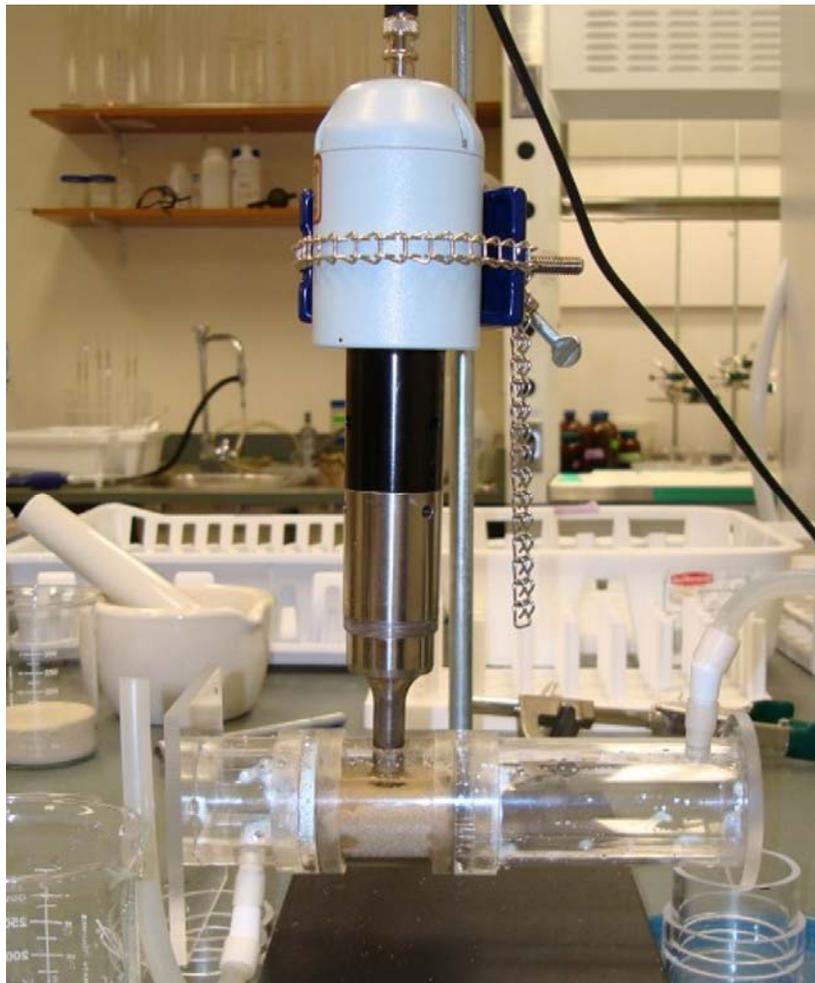
**Figure 3.6 Ultrasonic enhanced soil washing treatment system**
