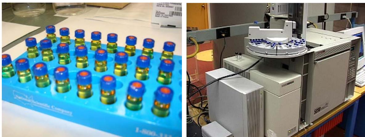
**Figure 3.10 GC-FID analysis; left: analysis vials; right: GC-FID analyzer.**
