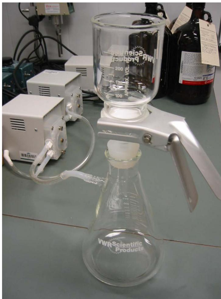
**Figure 3.3 Sample filtration apparatus setup**
