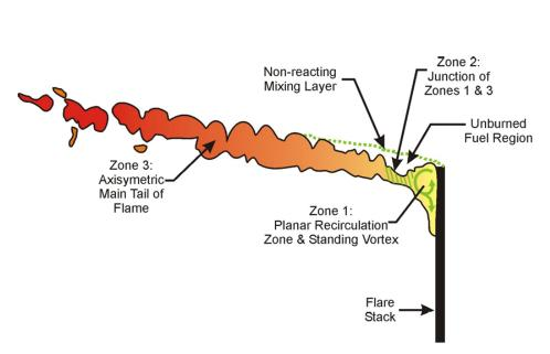
Figure 2.1 Flame Representation for a Flare in a Crosswind\*
