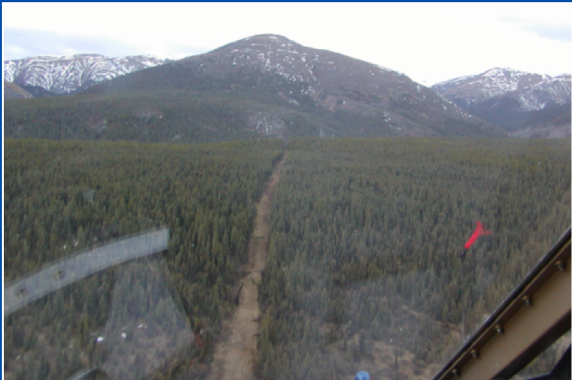
Use of existing cutline for access reduces footprint in the region. Cutline is very wet due to placement through forested wetland.
