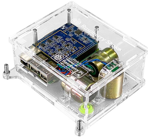
Figure 1: Image of a Raspberry Shake 3D seismograph. From <https://raspberrysshake.org/>
