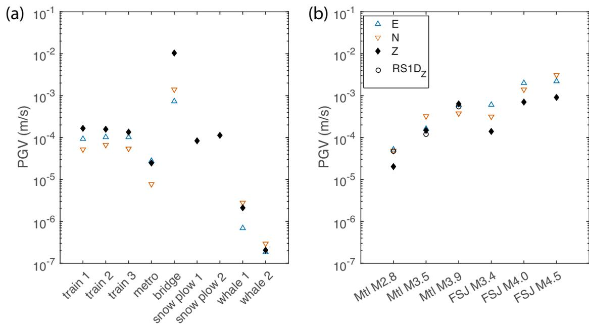
Figure 13: Summary of PGVs from (a) cultural and biological noises, and (b) tectonic and induced earthquakes. Three-component PGVs (E, N, Z) are shown if available. Open circle in (b) are Montreal earthquake PGVs recorded by the RS1D sensor R74C6.
