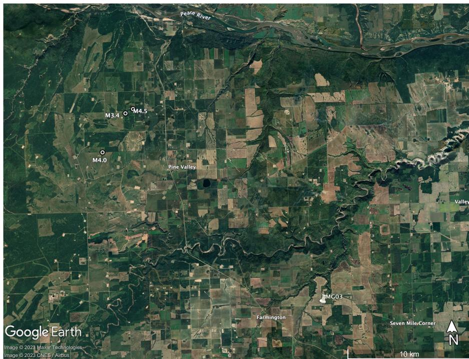
Figure 4: McGill station MG03 at (55.912151, -120.44136) recorded 2018-11-30 M4.5 hydraulic fracturing induced earthquake and its two aftershocks M3.4 and M4.0. White circles: epicenters of the three events.
