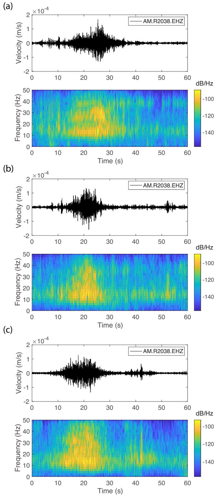
Figure 6: Waveforms and spectrograms of three examples of trains passing by seismograph R2038 (RS3D). (a) Train 1, distance of 20 m. (b) Train 2, distance of 25 m. (c) Train 3, opposing trains of distances 25 and 30 m. <sup>9</sup>
