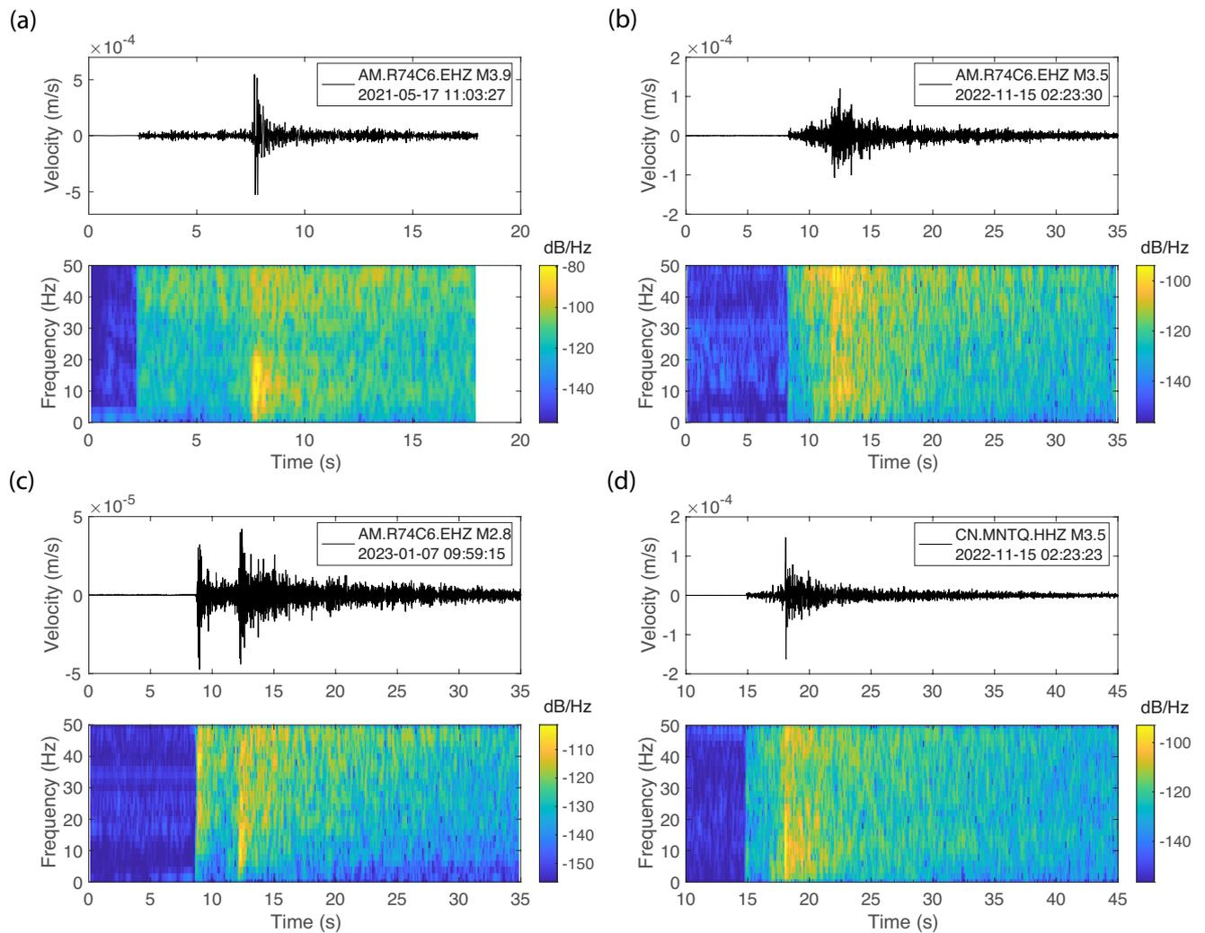
Figure 11: Velocity waveforms and spectrograms of (a-c) 2021-05-17 M3.9, 2022-11-15 M3.5, 2023-01-07 M2.8 earthquake near Montreal, recorded by the RS1D station R74C6 in NDG. (d) 2022-11-15 M3.5 earthquake, recorded at NRCan station MNTQ.
