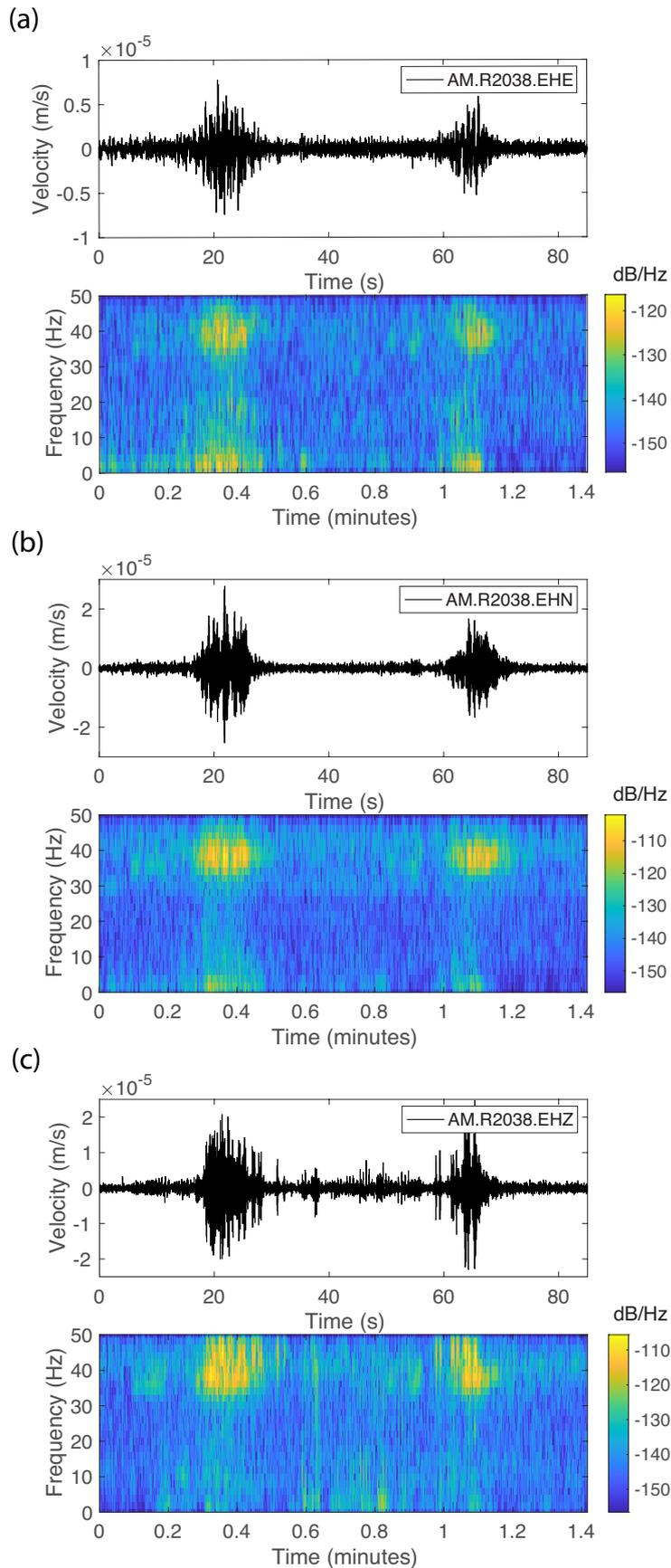
Figure 7: Waveforms and spectrograms of a metro train stopping and departing from the McGill metro station, recorded by R2038 (R53D). Measurement on platform,  $\sim 5$  m from the train. (a-c) East, north and vertical components, respectively. Note the x-axes for the spectrograms in minutes are aligned with the x-axes in seconds for the waveforms. Total recorded duration is 85 seconds.
