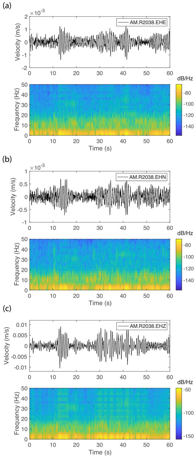
Figure 8: Waveforms and spectrograms of three components recordings by seismograph R2038 (RS3D) of traffic across the Jacques-Cartier Bridge, measured at the along-side bike path with source/receiver distance of 5-10 meters. (a-c) East, North and Vertical components, respectively.
