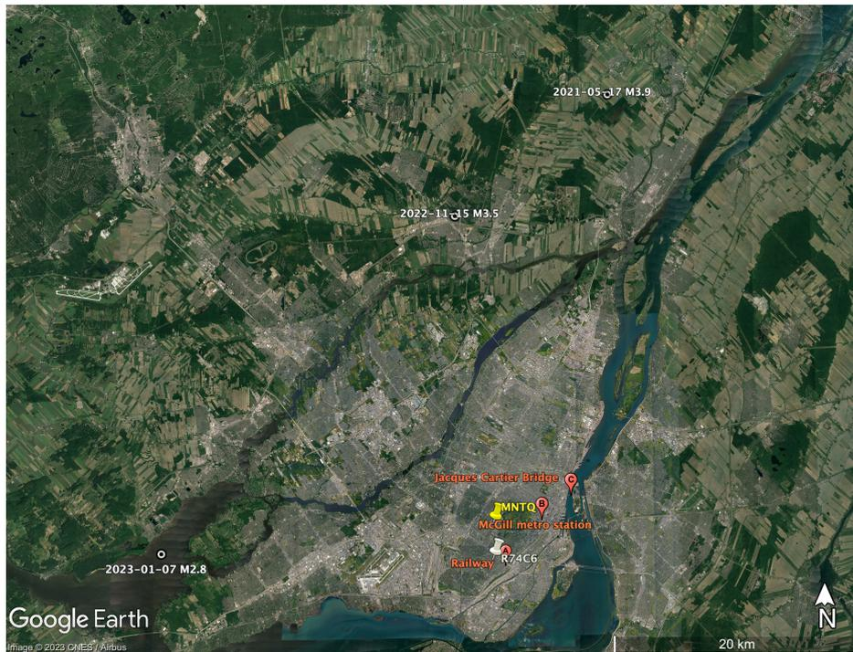
Figure 2: Locations of cultural noise recordings and tectonic earthquakes in/near Montreal. White pin: 1D Raspberry Shake (RS1D) station at a NDG basement (R74C6). Red balloons: mobile deployments in Montreal. A. near rail tracks, B. at McGill metro station platform, C. on the Jacques Cartier Bridge. White dots: epicenters of three recent tectonic earthquakes (details in Table 1).
