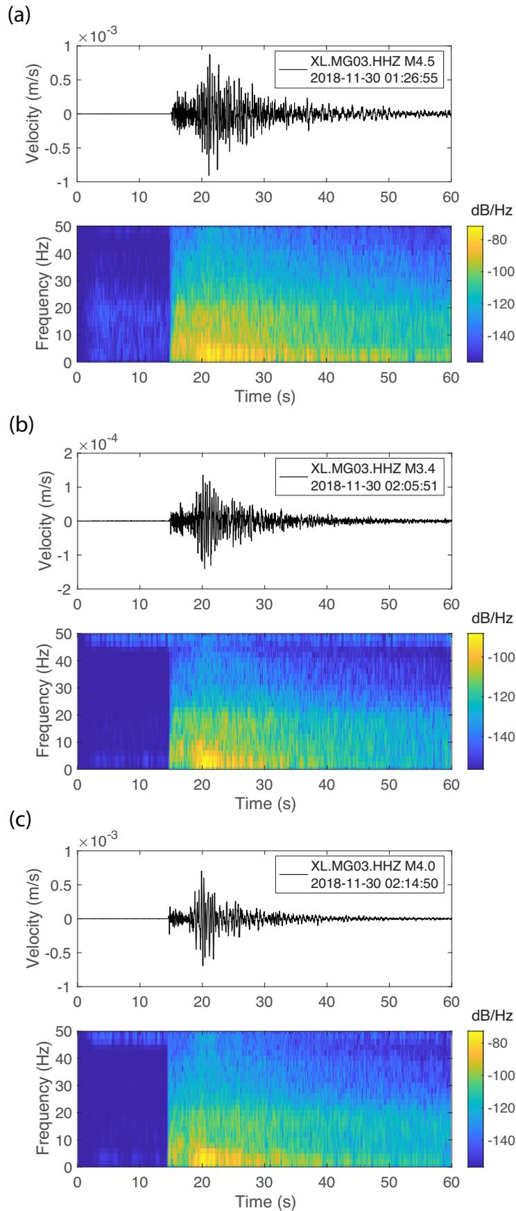
Figure 12: Velocity waveforms and spectrograms of (a) a M4.5 hydraulic fracturing induced earthquake near Fort St John on 2018-11-30<sup>17</sup> and its (b) M3.4 (c) M4.0 aftershocks on the same day, recorded at station MG03 about 20 km from the earthquakes.
