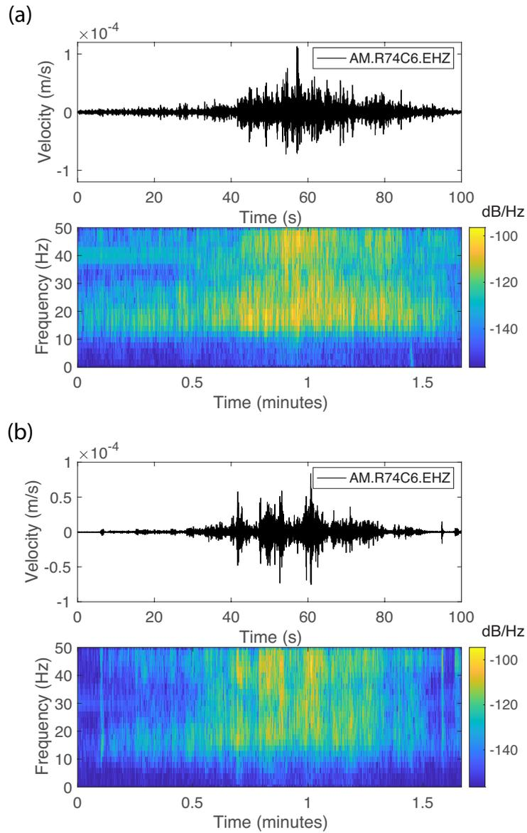
Figure 9: Waveforms and spectrograms of two recordings by seismograph R74C6 (RS1D) of snow plow driving by a family house in NDG, Montreal, in December 2022. Vertical component only. (a) Origin time 2021-12-08 11:42:40, UTC. (b) Origin time 2022-12-21 03:58:30, UTC.
