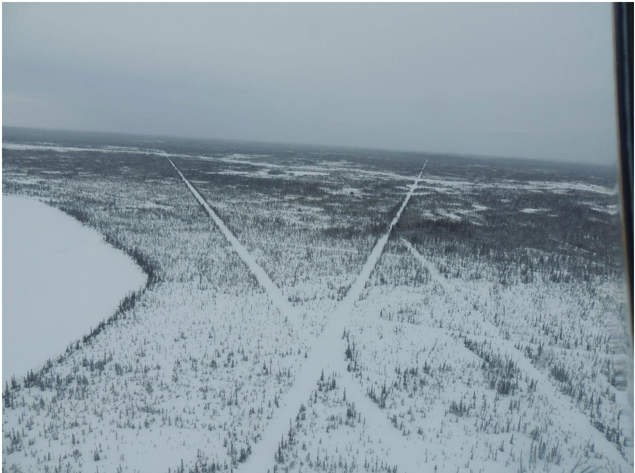
Figure 6. Often many low-impact seismic (LIS) lines recover more quickly than conventional lines and require less active restoration intervention. However, many LIS lines within the Medzih'tene Restoration Area (MRA) are "original style" LIS lines; they are quite wide and show very poor recovery success. In this case the two lines in the mid-ground orientated L-R are early LIS lines and still appear to contribute to wolf movement and increased caribou predation risk.
