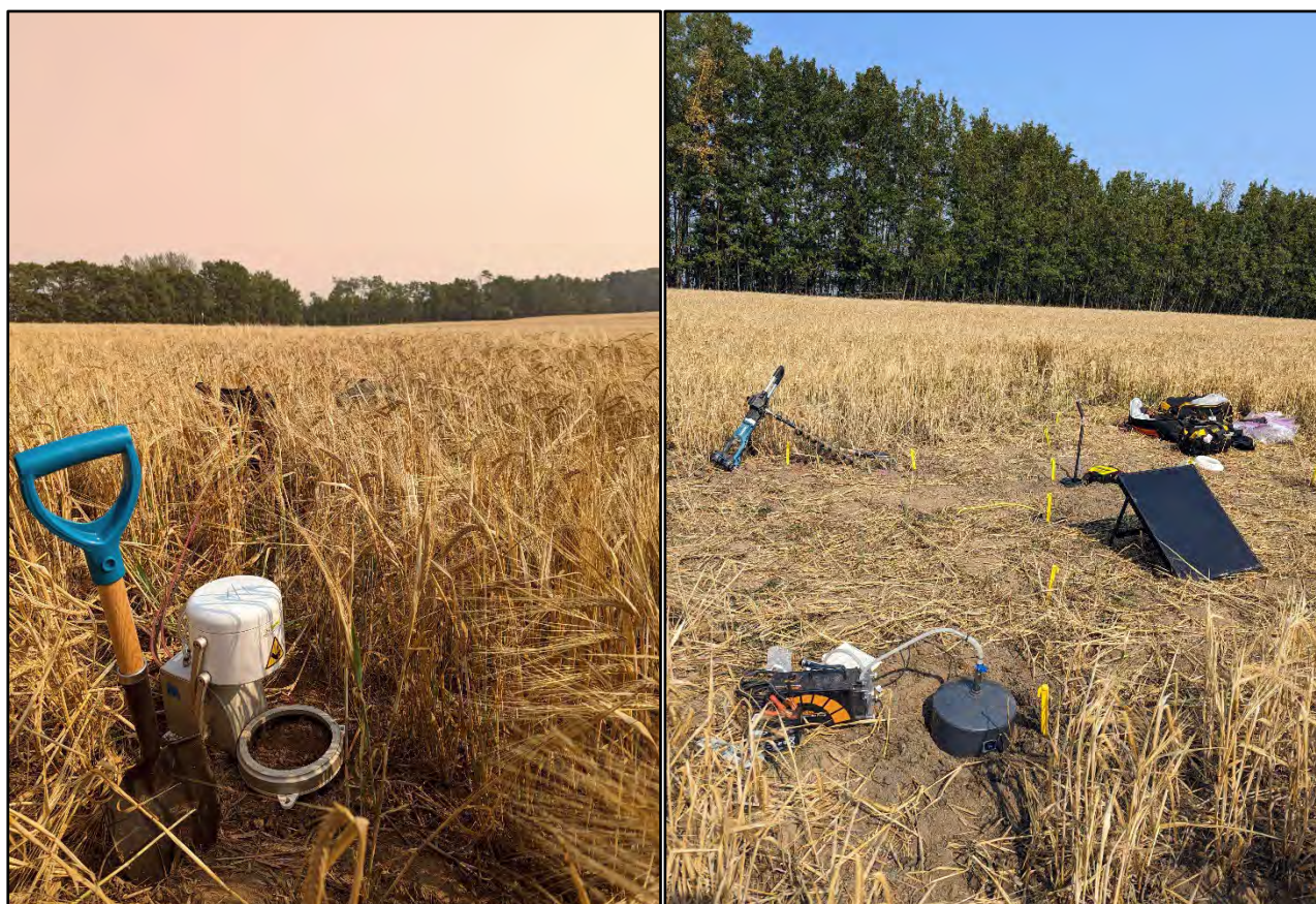
Figure 5: Dynamic (left) and static (right) flux chamber systems deployed during field investigations undertaken in 2023 at wellsite WA22800.
