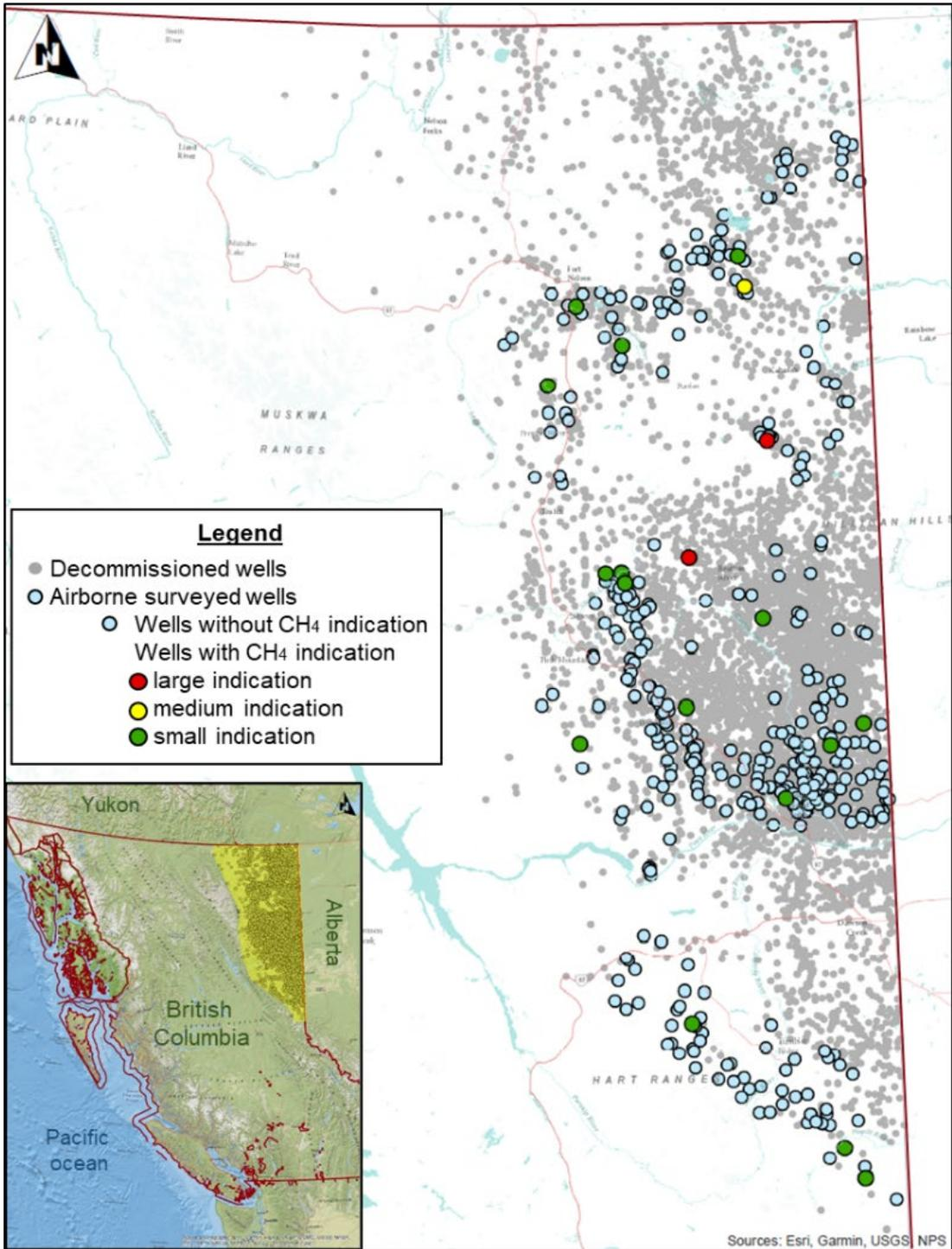
**Figure 5:** Map of BC showing decommissioned wells surveyed with airborne methods including both CH<sub>4</sub> detects (and indicative size) and non-detects as well as all currently P&A wells in the region (as small grey circles). The overall study area is highlighted (yellow) in the index lower left-corner map.
