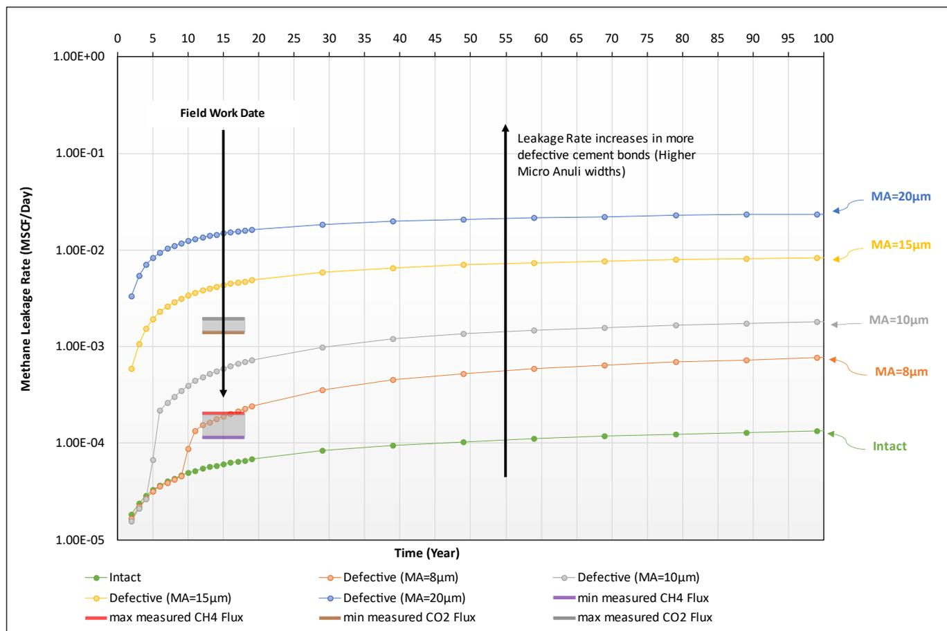
**Figure 9:** WA 22800 simulated potential leakage rates for varying MA scenarios with time. It should be noted that 1.00E-01 MSCF is equivalent to approximately 3 m<sup>3</sup>.
