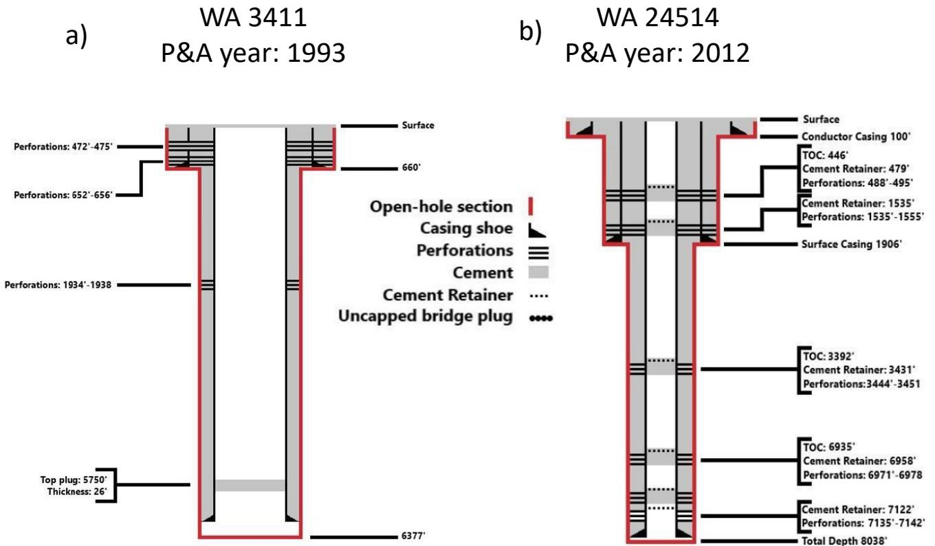
**Figure 2:** Example of 2 P&A configurations for decommissioned wells in BC of differing vintage, including; a) WA 3411, a gas well completed in 1976 and produced until 1988 before being abandoned in 1993. b) WA 24514, a gas well completed in 2009, going into production the same year before being P&A’d three years later in 2012.
