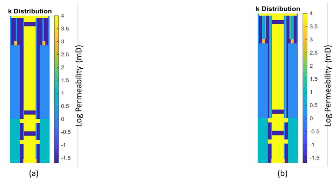
**Figure 7:** WA 22800 Well P&A Model Permeability Distribution: (a) Intact scenario with full integrity (b) Defective scenario with micro annuli of 13 μm between cement and casing representing the defect.
