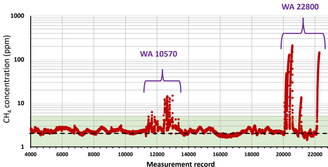
**Figure 7:** Concentration of CH<sub>4</sub> as measured with the flux chamber system during the whole field investigation campaign (i.e. throughout all site visits for both open and closed chamber status). The green shaded area shows the typical maximum natural range at which CH<sub>4</sub> may be detected in most natural environments relevant to NE BC. Results show CH<sub>4</sub> was typically low in concentration at all sites with the exception of WA 10570 and WA 22800.
