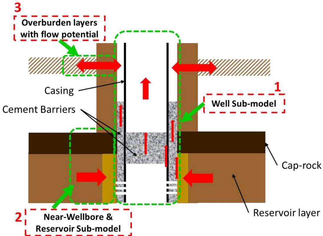
**Figure 1:** A schematic diagram of the integrated P&A system made up of three sub-models. The arrows indicate the potential flow/leakage pathways for hydrocarbons <sup>45</sup>
