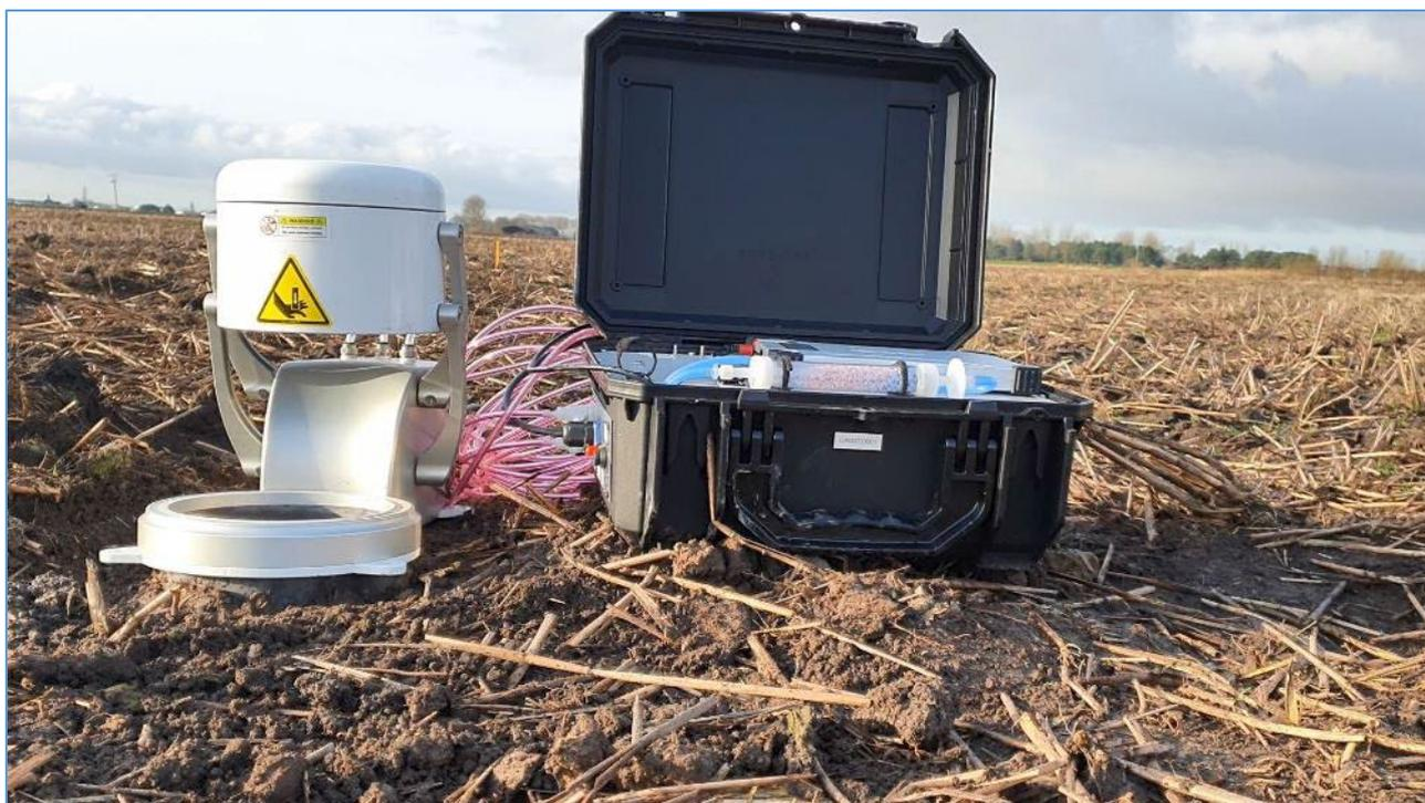
**Figure 5:** Dynamic flux chamber system deployed during field investigations showing the chamber unit installed on a collar connected to the analyzer unit.
