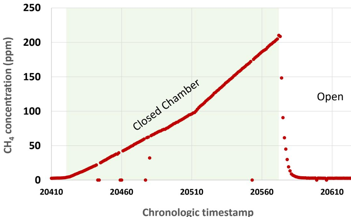
**Figure 8:** Concentration of CH<sub>4</sub> with time during a single flux measurement taken at the wellhead center of WA 22800. Results show a clear, stable and significant increase in CH<sub>4</sub> from background levels to > 200ppm during the closed chamber period of 5 minutes, generating an associated flux estimate of 3 μmol/m<sup>2</sup>/sec (compared to a background estimate of -0.03 μmol/m<sup>2</sup>/sec attained some 50 m away in the same crop field).
