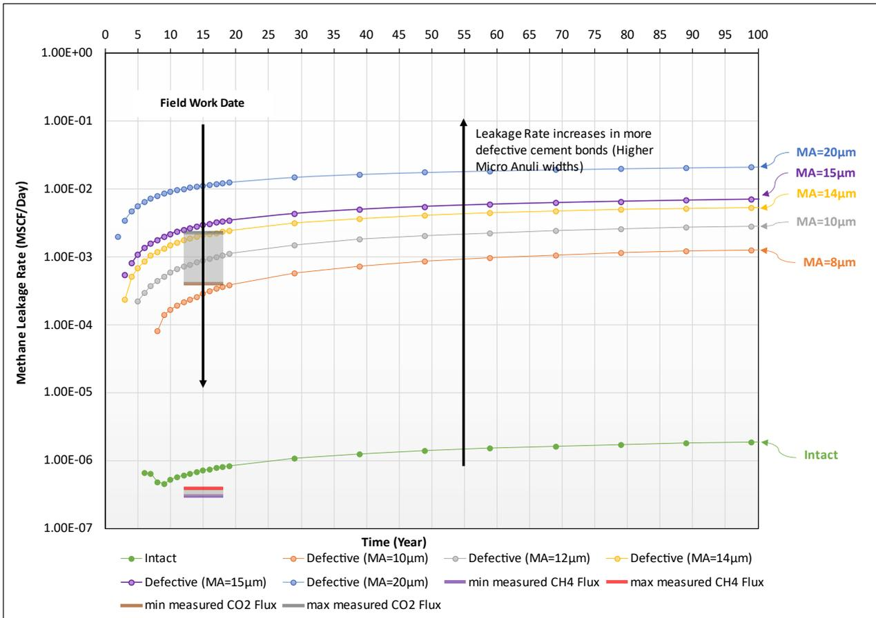
**Figure 10:** WA 21083 simulated potential leakage rates for varying MA scenarios with time. It should be noted that 1.00E-01 MSCF is equivalent to approximately 3 m<sup>3</sup>.
