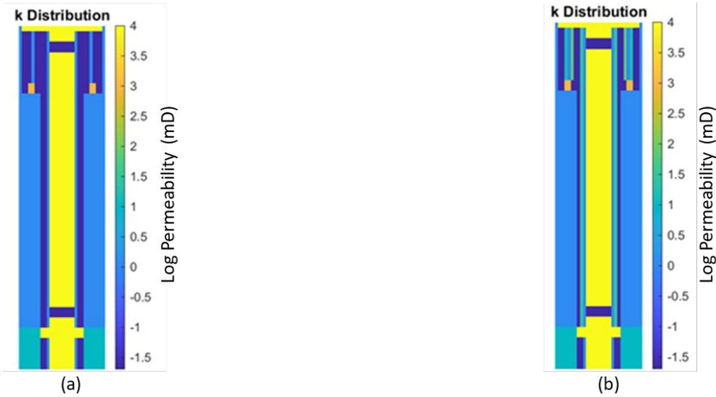
**Figure 8:** WA 21083 Well P&A Model Permeability Distribution: (a) Intact scenario with full integrity (b) Defective scenario with micro annuli of 13  $\mu\text{m}$  between cement and casing representing the defect.
