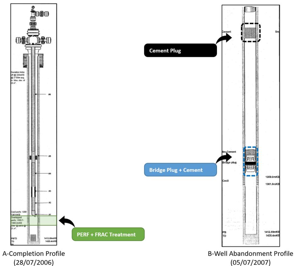
**Figure 6:** Completion (A) & Abandonment Design (B) for WA 21083
