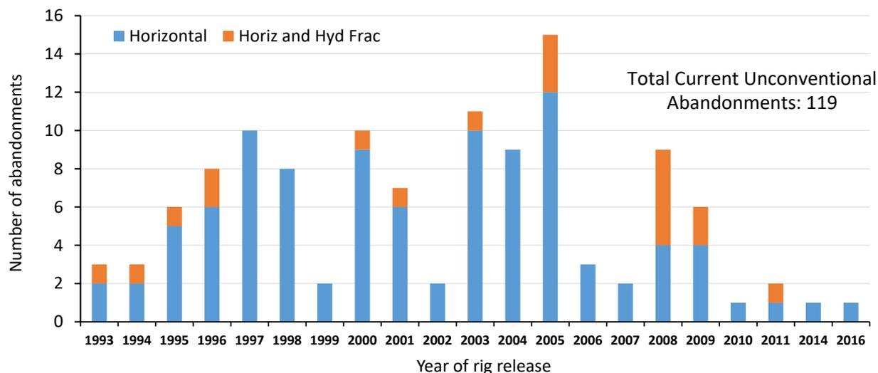
**Figure 1:** Histogram showing number of existing P&A’d unconventional wells in BC (a total of 119 out of population of 7600) by rig release year including proportions of horizontal only (a total of 100 wells) and horizontal and hydraulically fractured wells (a total of 19 wells).
