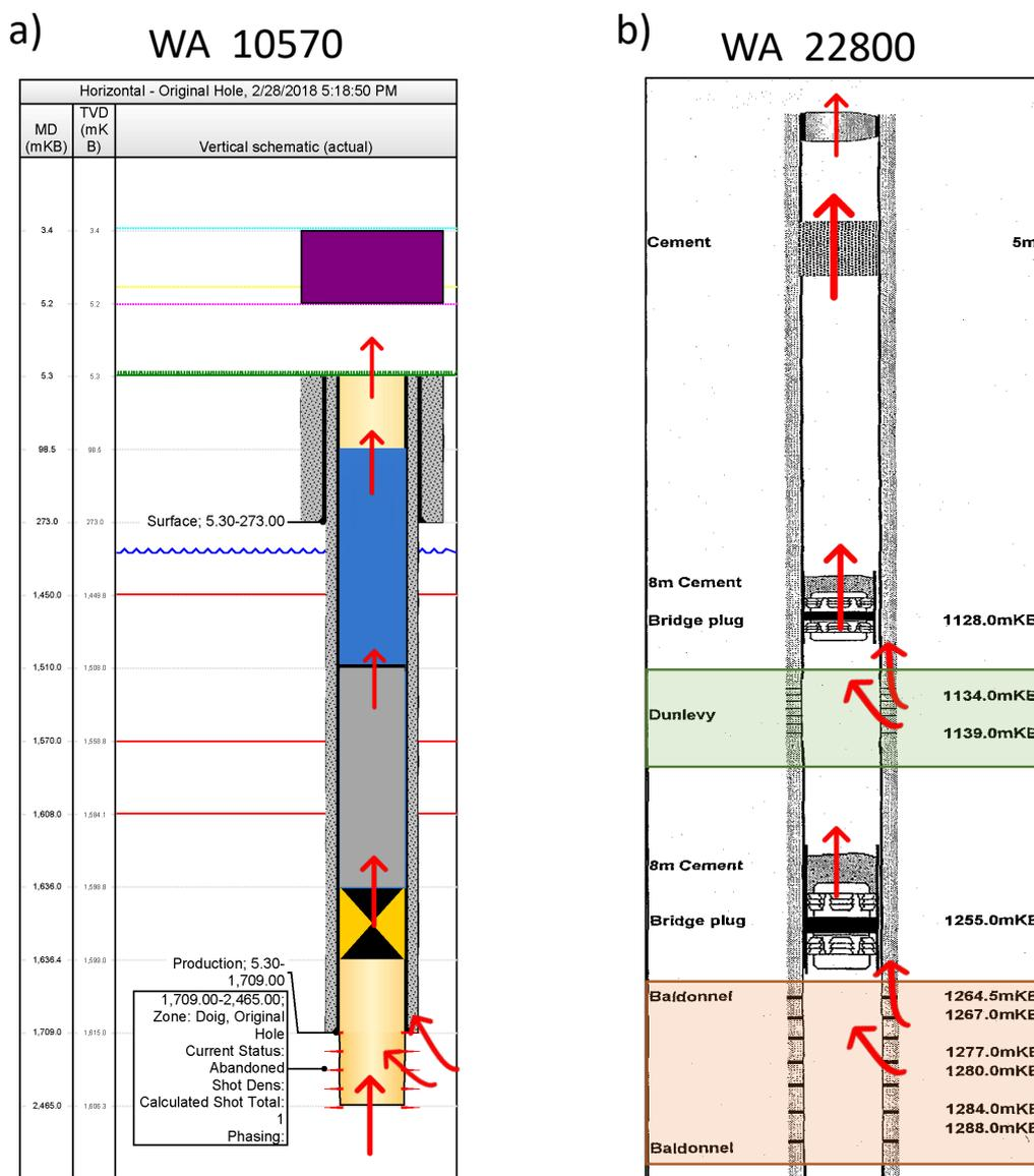
**Figure 14:** Well completion and P&A schematics for wells identified as potentially suffering integrity failure during field investigations, including potential fugitive fluid migration pathways indicated by red arrows.
