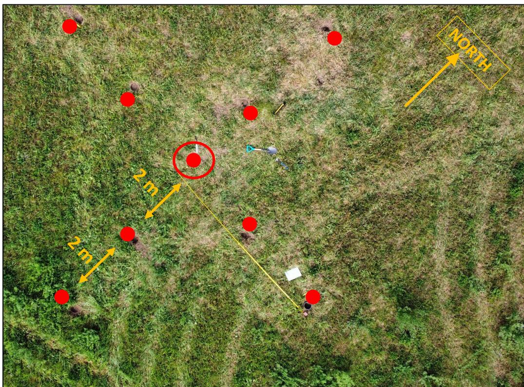
**Figure 3:** Monitoring grid deployed at each wellsite showing the 9 monitoring points in a cross hair configuration, oriented North, covering an area of 8 m<sup>2</sup> (2 m distance between each point) and centered over the assumed wellhead.
