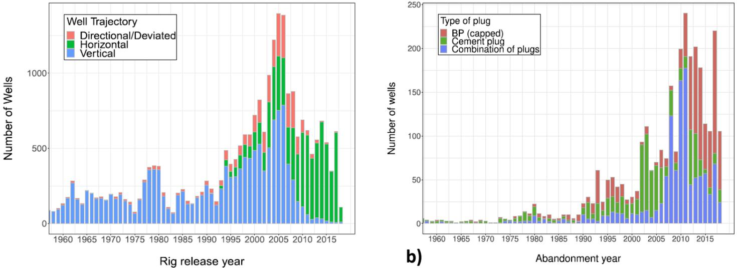
**Figure 1: a)** From Trudel *et al.* (2019). Wells released per year in BC showing the significant upturn in unconventional development. **b)** P&A’s per year in BC and type of plug utilized showing varying configurations, an increasing number of abandonments and increased use of bridge plugs.
