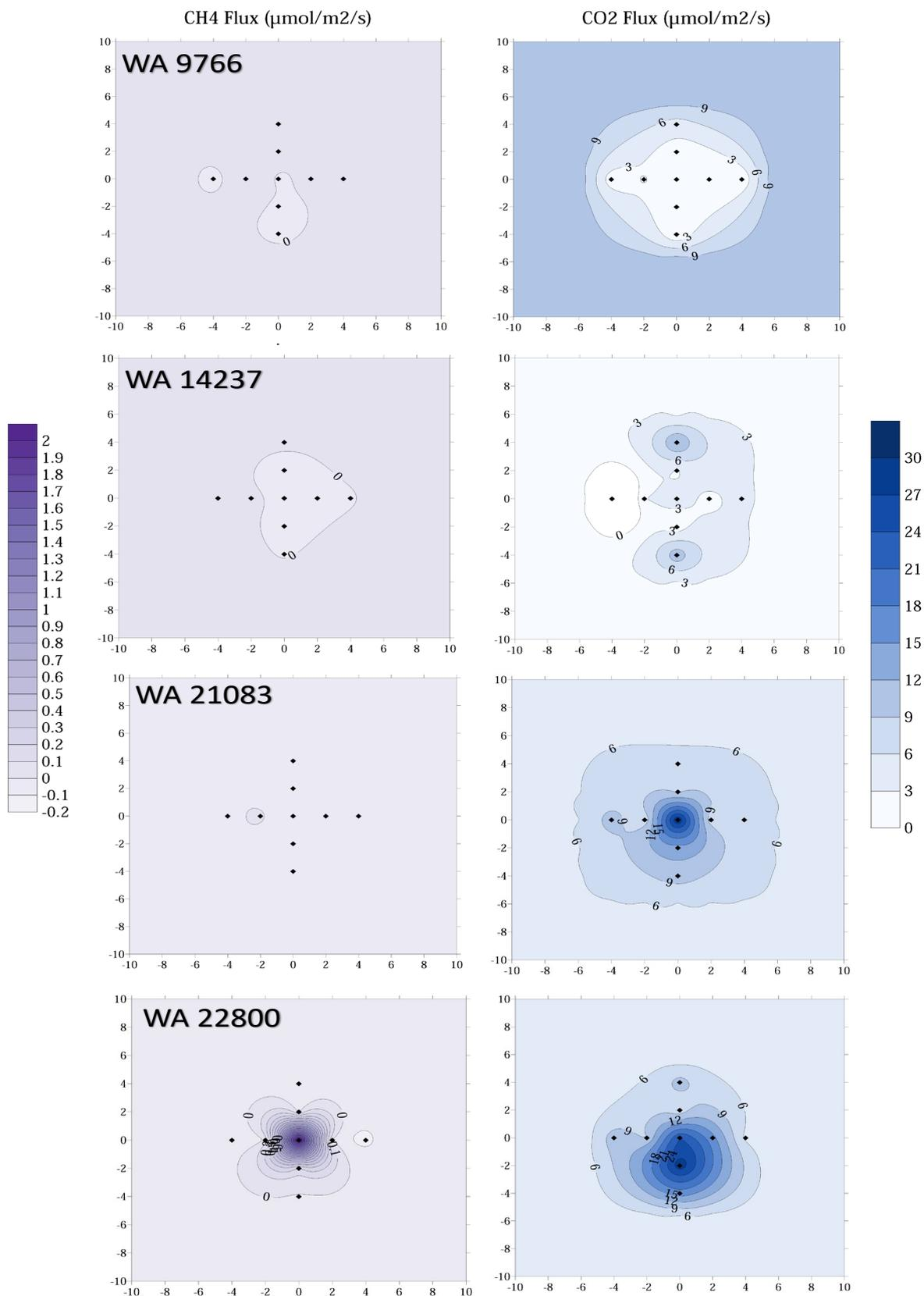
**Figure 9:** Plan view contour plots of CH<sub>4</sub> and CO<sub>2</sub> flux (interpolated by Krigging) as calculated from rates of change in concentrations detected with the dynamic flux chamber system for select investigated P&A'd well sites.
