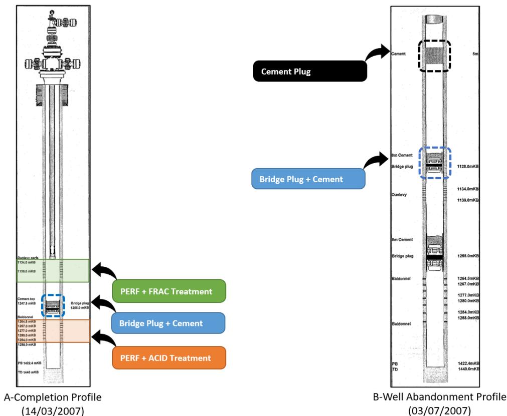
**Figure 5:** Completion (A) & Abandonment Design (B) for WA 22800
