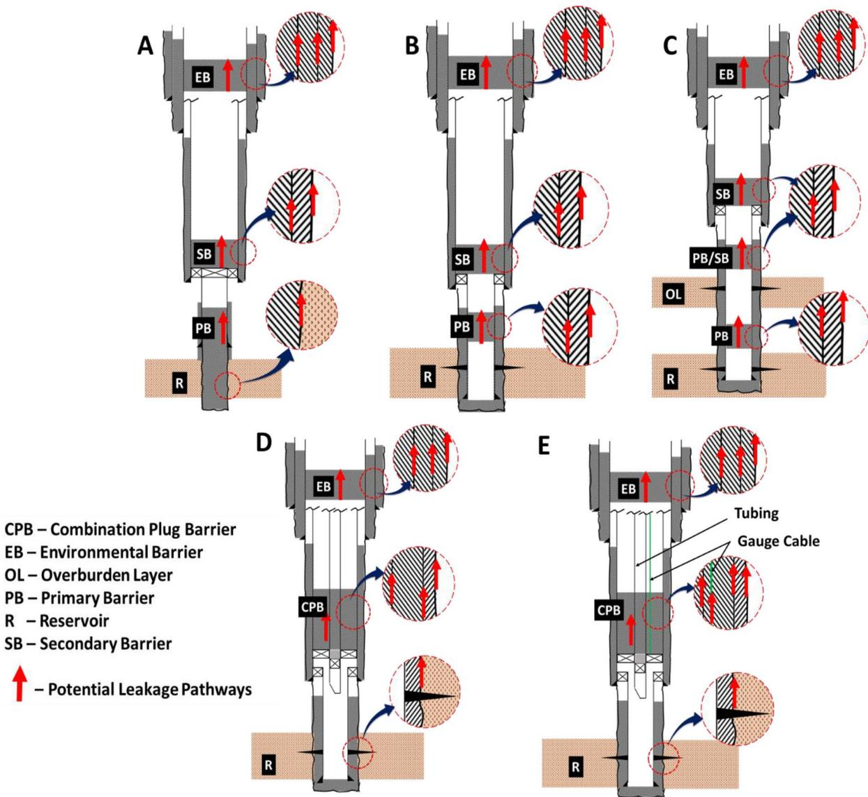
**Figure 2:** P&A Design scenarios covered by the P&A modelling framework: A) open-hole, single layer, B) cased-hole, single-layer, C) cased-hole, multi-layer, D) through-tubing abandonment without gauge cable and/or hydraulic line E) through-tubing abandonment with gauge cable and/or hydraulic line <sup>45</sup>.
