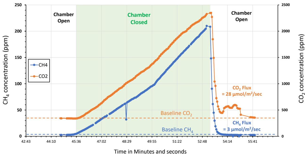
**Figure 13:** CH<sub>4</sub> and CO<sub>2</sub> concentrations observed during a flux measurement at wellsite WA 22800 showing co-emission indicative of CH<sub>4</sub> oxidation occurring in the surrounding soils.
