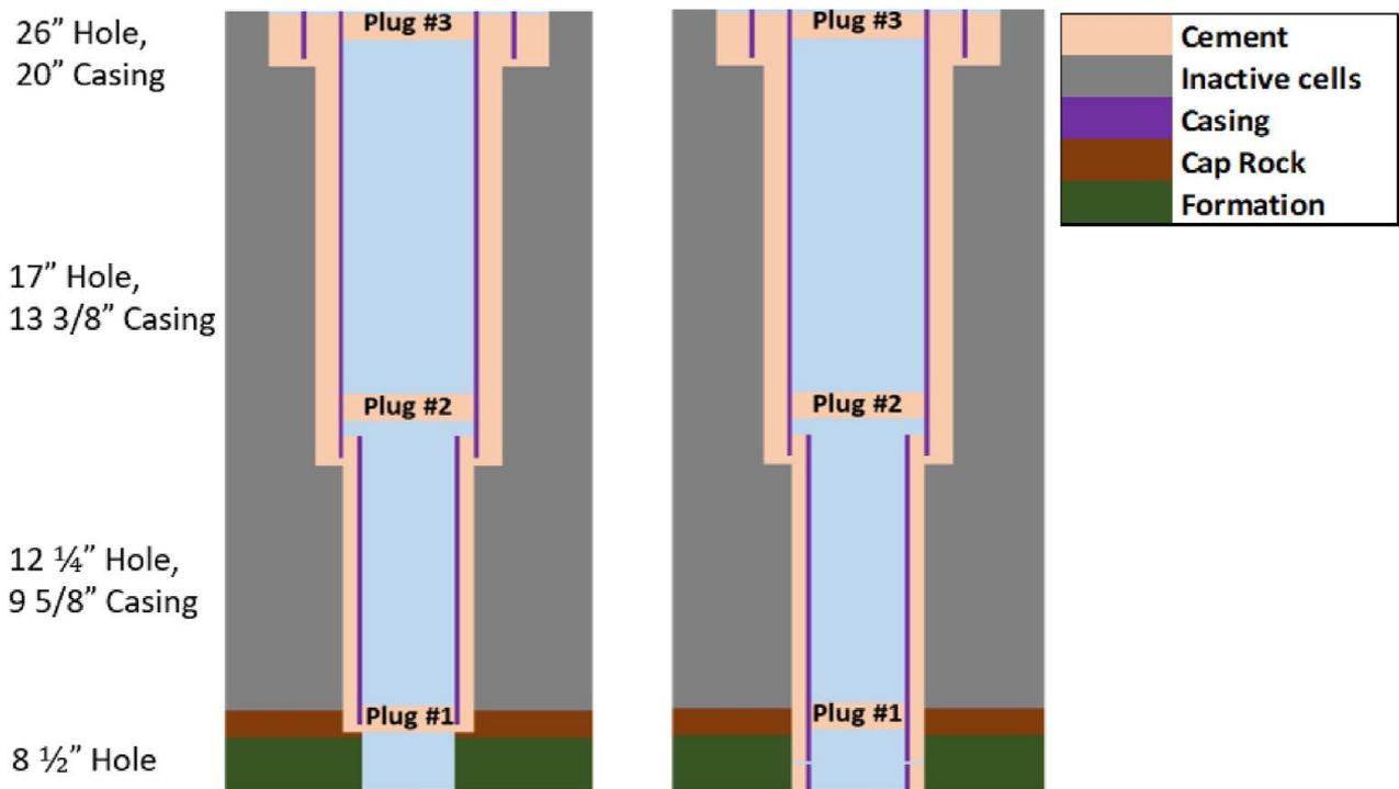
**Figure 3:** Well schematics for a multiple-plug (Left) open-hole P&A scenario and a (Right) cased-hole P&A scenario <sup>45</sup>
