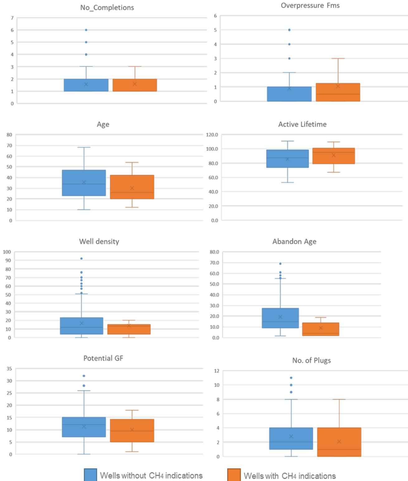
**Figure 8:** Example of box and whisker plots for CH<sub>4</sub>-detect and non-detect wells that were identified during the aerial surveys showing distribution of parameters including equivalency (e.g. no. of completions) and what appear to be significant differences (e.g. abandonment age).
