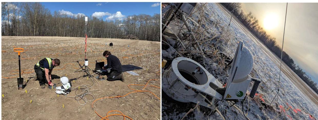
Figure 3: Fieldwork at Wellsite J during the April/May (left) and November (right) 2025 Phase 3 campaigns. The images show contrasting field conditions during the two dedicated campaigns, including flux monitoring and shallow soil sampling around the leakage hotspot. Together, these campaigns extended the observational record beyond previous summer-focused work and generated the multi-domain dataset used to support Phase 3 interpretation.
