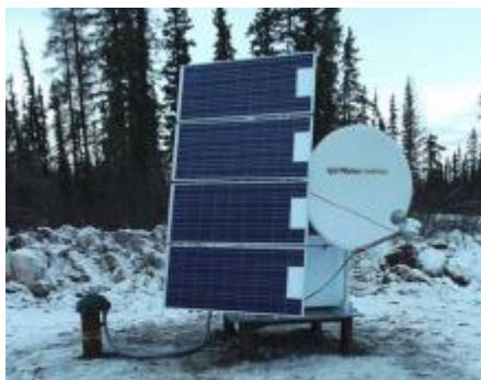
Northeast B.C. Seismic Array Network Project—an installed seismograph station (courtesy Geoscience BC).
