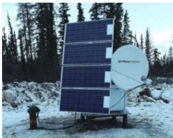
Seismic Array Network project equipment—an installed seismograph station (courtesy Geoscience BC).
