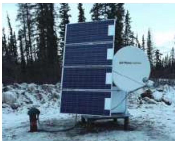
Seismic Array Network project equipment—an installed seismograph station (courtesy Geoscience BC).
