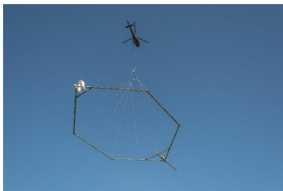
Aerial Equipment Mapping Groundwater Aquifers in the Peace Region (courtesy Geoscience BC).
