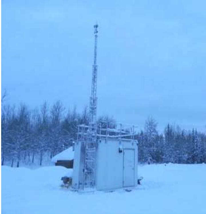
**Figure 2** The new air quality station at Doig River. All three of the new air quality stations were installed in December 2013 and monitor sulphur dioxide (SO<sub>2</sub>), total reduced sulphur (TRS) and meteorology including air temperature, relative humidity and wind speed and direction).
